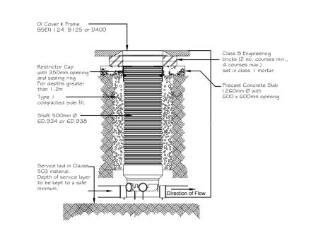
08 FOUL SEWER INSPECTION CHAMBER (F.I.C)
