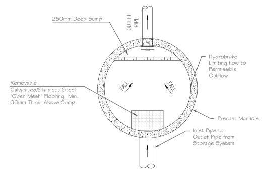
O4 Typical Plan of Hydro-Brake Manhole
