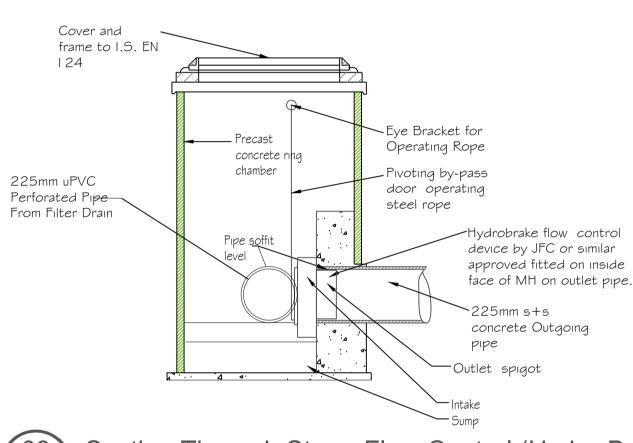
Section Through Storm Flow Control (Hydro-Brake) Manhole SCALE 1:50
